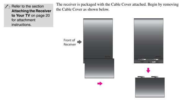
Gently slide the Cable Cover toward the rear side of the receiver, then pull down.
